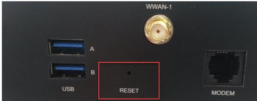
This inset reset button allows you to reset the IOLAN or reset the IOLAN to the Perle factory default settings.
