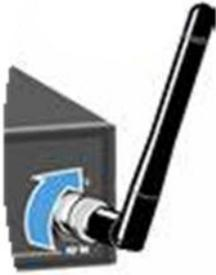
**Note:** When attaching the antennas to the SMA connectors hand tighten only (do not use tools to tighten (maximum torque is 7Kgf-cm/1.1 N-m(10 in-lb)).
