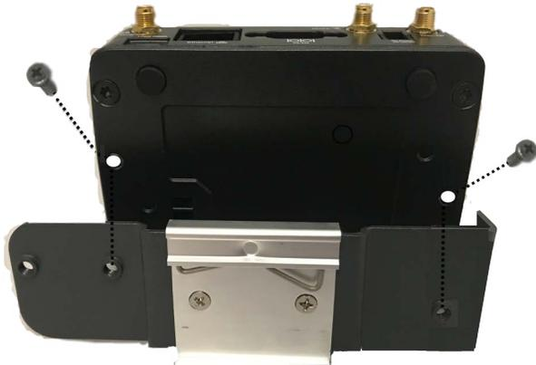
3. Position the router such that the top hooks of the DIN rail clip attach onto the top of the DIN rail.
