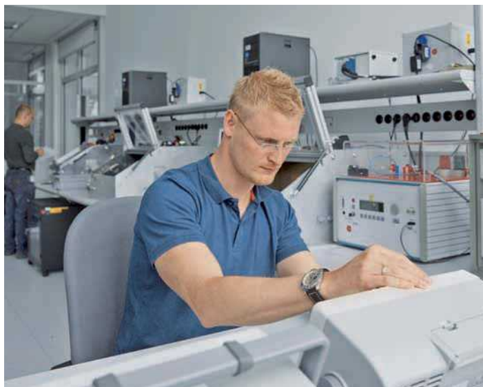
Fig. 25: Fully automated testing system for determining the overload and failure behavior of surge protective devices according to IEC 61643-11 [6]
