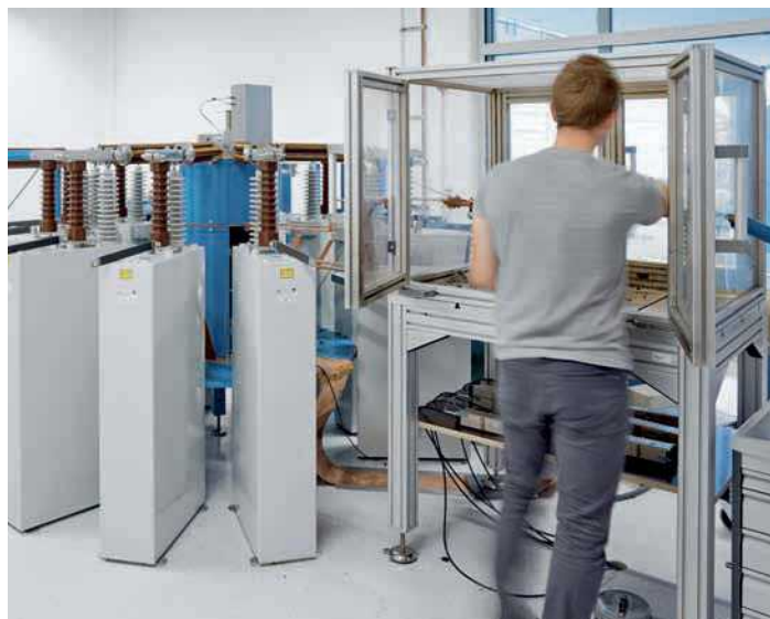
Fig. 26: Lightning surge current generator
