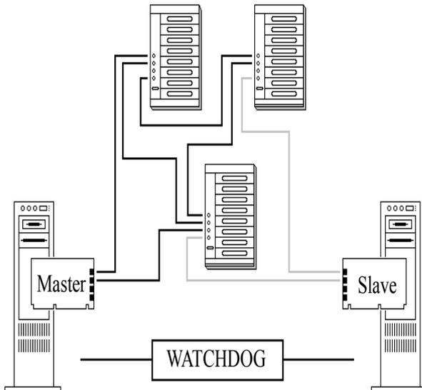
In master/slave mode, the slave host exists solely to provide support for the master system.
