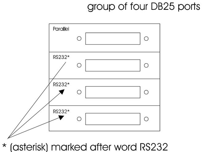
**Note:** As an option you can have order the RS232\* ports with surge suppression capability. This feature allows the ports to absorb high static discharges and surges.
