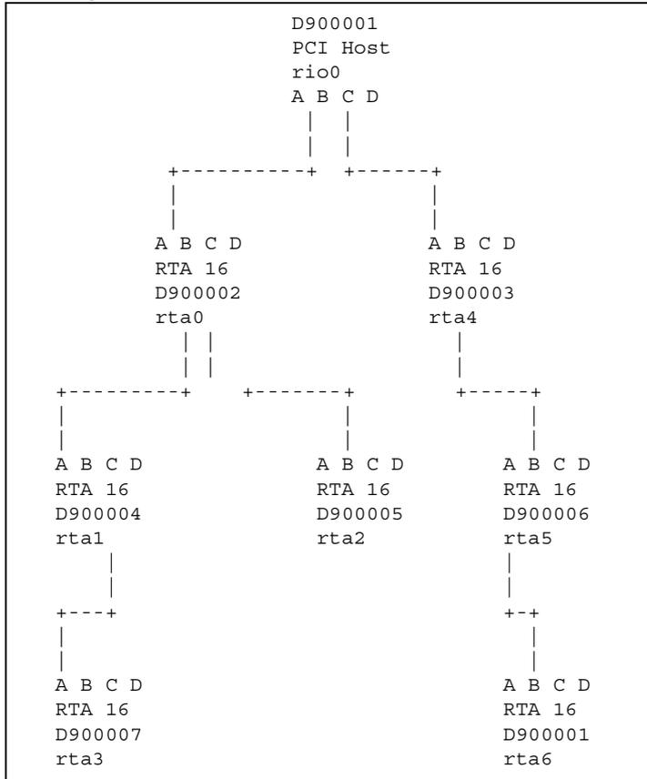
**Note** *If you have fault tolerant links installed, your RTA Topology may not look how you expect. See Section 7.2 Adding a Fault Tolerant Link.*
