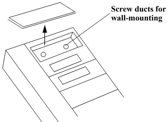
**Note** *When installing RTAs, particularly if wall-mounting, make sure that you follow the correct strain relief procedures in order to avoid undue strain on RIO link connection*
