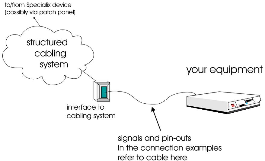
2. *Within* the structured cabling system, we presume you use straight-through cabling, i.e. pin 1 to pin 1, pin 2 to pin 2, etc.
