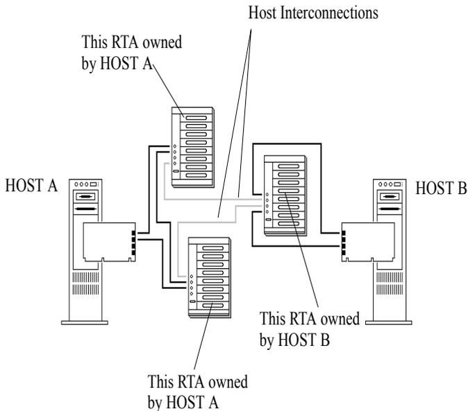
1. Install host card A, connect and configure the RTAs that you want owned by host A. Using fault tolerant links, make sure each RTA has at least one route to the host card.
