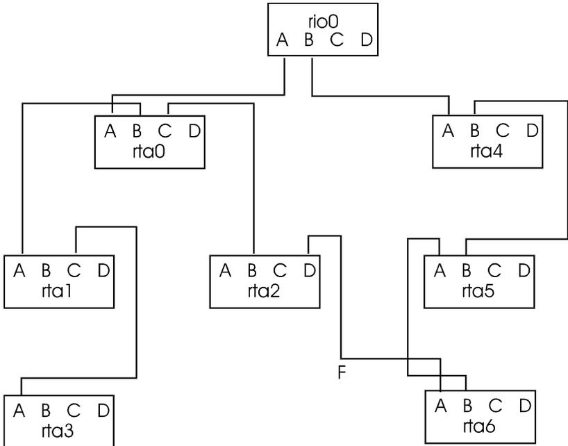
The fault tolerant link has effectively connected Links A and C on the host card. When the topology gets to rta2, it now finds link D connected to rta6 and so on. The RTA network connected to Link C will now be treated as an extension to the RTA network connected to Link A.
