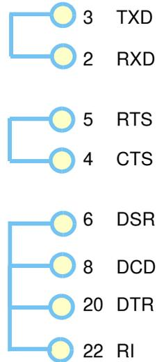
For details of DB25 female connector pinouts see [page 157](#).
