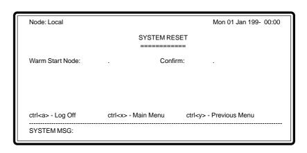
You have now successfully set up your local LINKSTREAM. Before configuring the remote unit, perform a system reset. This screen is entered to reboot the system and requires a confirmation response.
