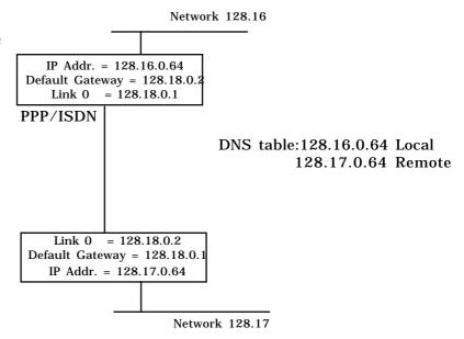
To manually configure the unit for the example above, follow through the configuration menus detailed on the following pages.
