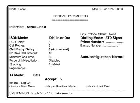
These parameters only need configuring if an ISDN interface is required.
