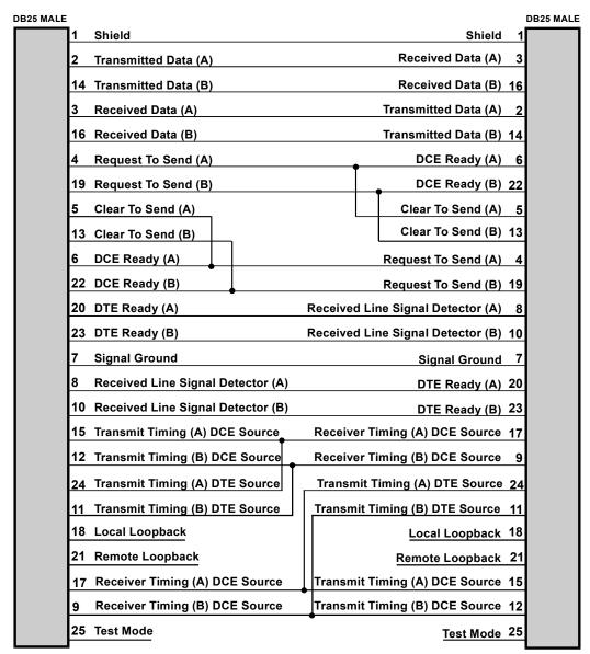
Figure C-13 RS530 / RS422 Null-Modem Cable
