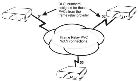
Figure 2 - 1 Frame Relay configuration
