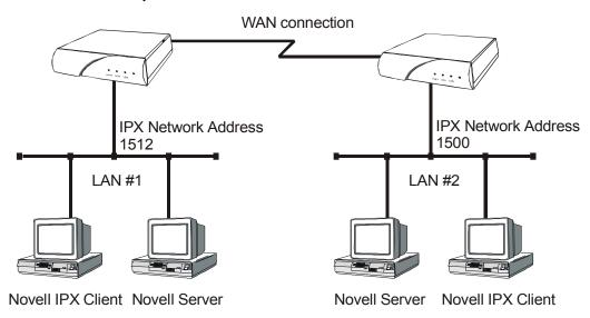
Figure 2 - 7 IPX Routed Local Area Networks (Servers on both sides)
