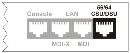
standard RJ45 service connector, pinout specification RJ48S.
