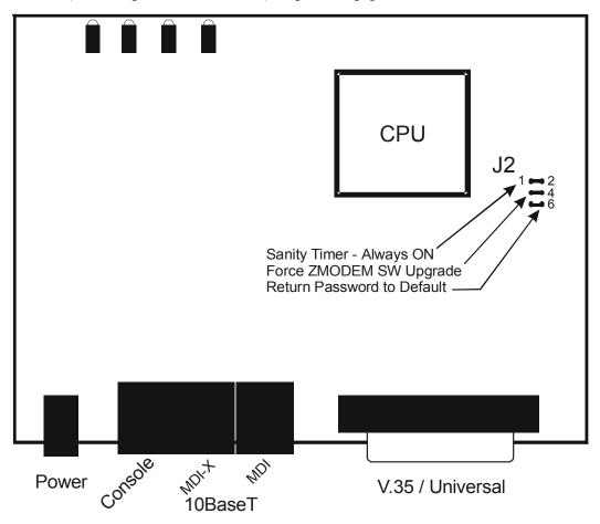
Figure C-1 Top Internal View of the P850 router V.35 or Universal WAN interface
