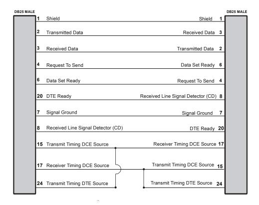
Figure C-12 RS232 / V.24 Null-Modem Cable
