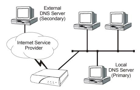
Figure 2 - 9 Local + External DNS Server Configuration
