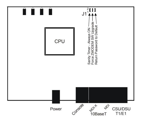
Figure C-2 Top Internal View of the P850 CSU-DSU or T1/E1
