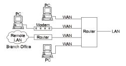
For IP, the 833IS looks like a router between two networks. The first network is comprised of the devices on the LAN. The second network, referred to as the "Internal WAN network", is comprised of all IP clients and routers that are dialed into the WAN ports.
