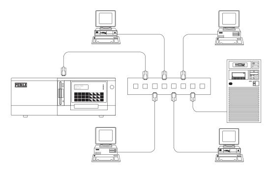
For a 10BaseT or 100BaseTX connection, the concentrator hub is connected as described in the vendor documentation. The Perle 594 may be connected to the concentrator hub using a 10BaseT Ethernet cable (see page 29).
