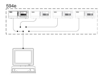
The Perle 594e can be configured to allow any NWS to access any session on any of the Multisession Controllers. The Perle 594e allows the user to switch the NWS from one session to another by pressing a "hot key" sequence.
