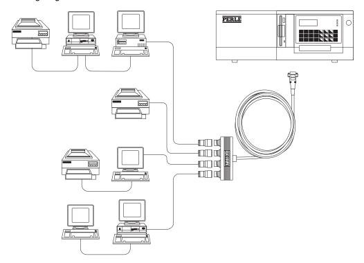
The Twinaxial Feature Card comes equipped with a Twinaxial Adapter Cable, which has four twinaxial connectors. A single twinaxial line can be attached to each connector.
