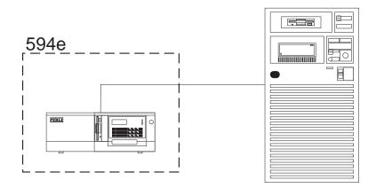
The Perle 594e can also emulate additional controllers without the need for additional Twinaxial or ASCII Feature Cards. The additional controllers are called Multisession Controllers. The system configuration will have the following appearance to the AS/400:
