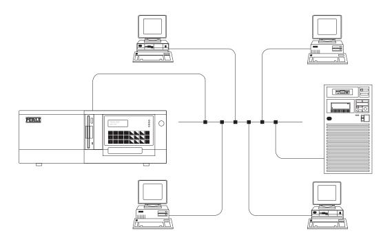
For a 10Base5 (Thick Ethernet) connection, the Perle 594 is attached to a transceiver on the network trunk using an AUI cable attached to the AUI port on the feature card (see page 28).
