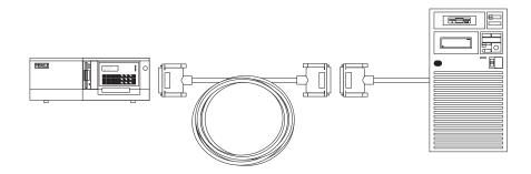
For V.35 cabling, the Perle 594 communication cable is equipped with a V.35 connector. The IBM AS/400 communication cable can be plugged directly into the Perle 594 communication cable.
