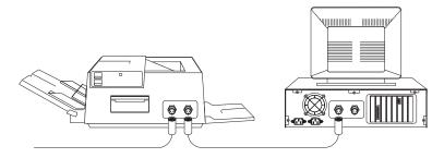
Instead of twinaxial cables, you may decide to use Telephone Twisted Pair (TTP) cables. TTP cable is less expensive than twinaxial cable. It is also smaller in diameter and is therefore easier to install. In many buildings, extra TTP cable was included when the telephone wiring was initially installed.
