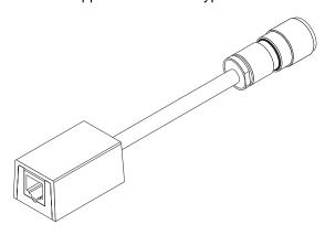
With TTP, each workstation must have its own TTP wire leading to a "hub". Depending on the vendor, a hub may have up to seven TTP connectors for the attachment of workstations. The connection to the Perle 594 is made with a single twinaxial cable. The following diagram shows the appearance of one type of hub.
