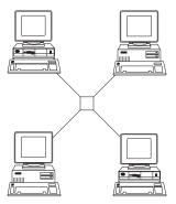
Each Ethernet Feature Card can support a maximum of 80 PWSs. The Perle 594e can support up to two Ethernet Feature Cards, for a maximum of 160 Ethernet PWSs.
