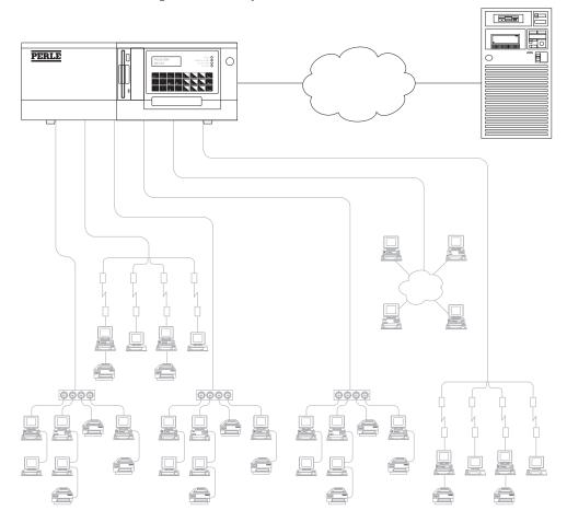
In Enhanced Mode the Perle 594e appears to the AS/400 as many IBM 5494 controllers sharing a multi-point communication line.
