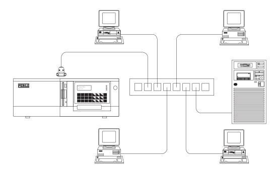
The MAU is connected as described in the vendor documentation. The Perle 594 may be connected to the MAU using the Perle-supplied Token-Ring cable.
