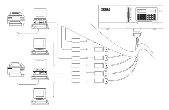
The ASCII Feature Card comes equipped with an ASCII Adapter Cable, which has eight (8) serial ports. A serial modem can be attached to each port, and a single user can dial-in to each modem. Up to eight (8) users can access the ASCII Feature Card simultaneously.
