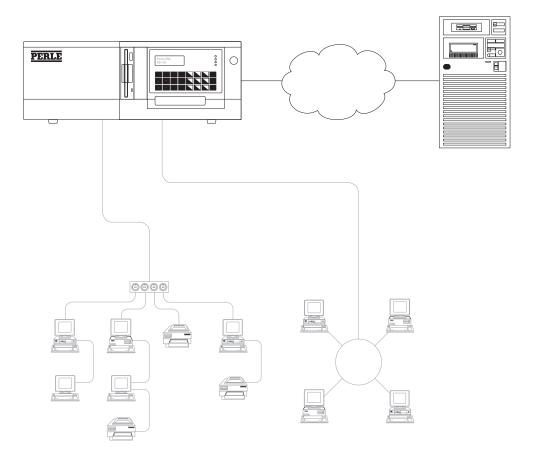
The Perle 594e (in compatible mode) appear to the AS/400 as single IBM 5494 controllers.
