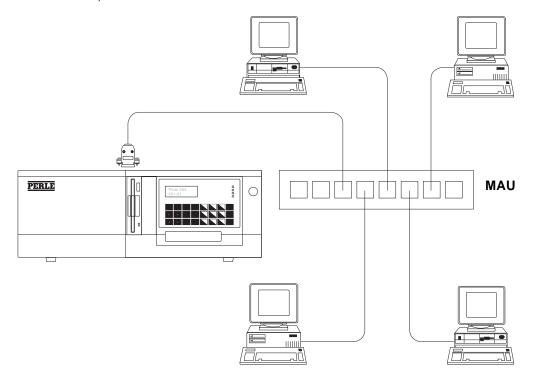
The connection between a device and the MAU is called a "lobe". Each device must be equipped with an "adapter", which is a circuit board or computer card that allows the device to attach to the lobe.
