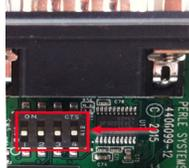
Note: For EIA-232 these switches must be in the OFF position (default)
