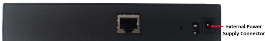
Plug the power adapter into a power socket and connect the barrel connector end into the IOLAN. The IOLAN will perform a power up sequence. The Power/Ready LED should show a solid green. See [LED Indicators](#) for power up sequence.
