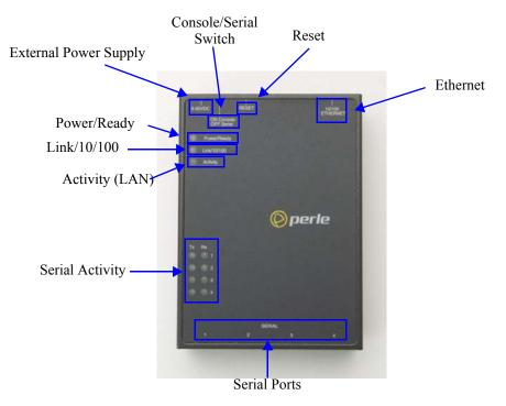
The 4-port IOLAN model has four RJ45 serial connections. The STS8-D IOLAN model has eight RJ45 serial connections. This sections describes the basic components found on the IOLAN I/O models.
