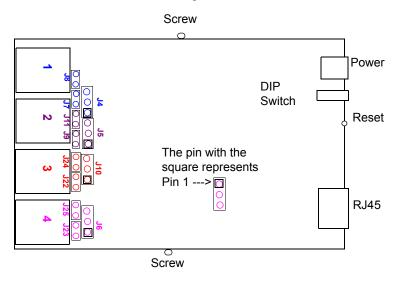
**3.** The following table describes how to jumper the pins for line termination, fixed 5V output, and for output equal to the external adapter input:
