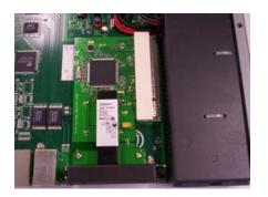
**10.** You can now replace the top of the IOLAN chassis by aligning it and sliding it into the base. You can throw away the face plate, as you will not be needing it.
