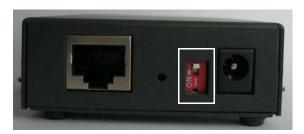
Look at your model to verify the direction of the ON switch position. ON indicates that serial port 1 is in Console mode; otherwise serial port 1 is in Serial mode.
