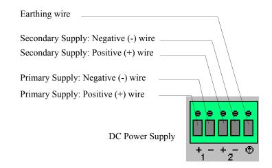
**Note:** When connecting only a single power supply source, ensure the connection is the primary supply and the secondary terminals are left unconnected.
