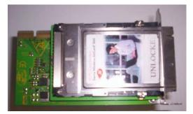
9. Slide the PCI adapter card into the PCI slot.
