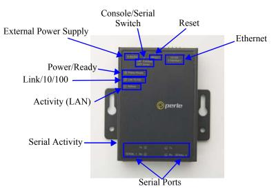
The 2-port IOLAN has two RJ45 serial connections. The 2-port IOLAN can support an 8-pin connector if there is no requirement for power in (pin 1) or power out (pin 10) pins. The 2-Port P model (Power over Ethernet) does not come with an external power supply connector.
