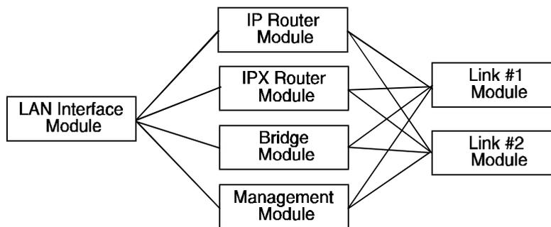
**Figure 1 IOLINK SOHO Ethernet Bridge/Router Block Diagram**
