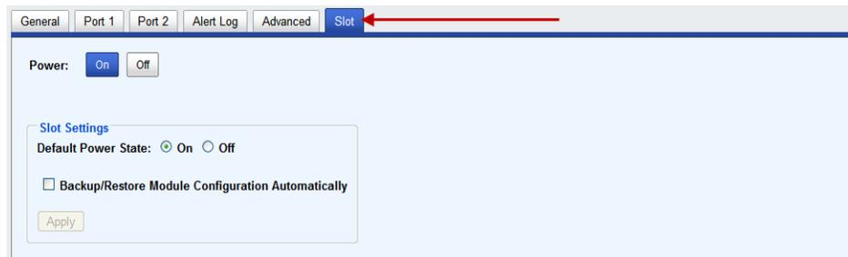
**Power State** Immediately power the slot on or off. The current state of the slot is highlighted in BLUE.
