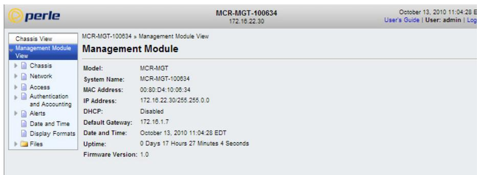
The main screen is divided into two sections. On the left is the “navigation tree” and on the right is the information associated with a specific selection on the navigation tree.
