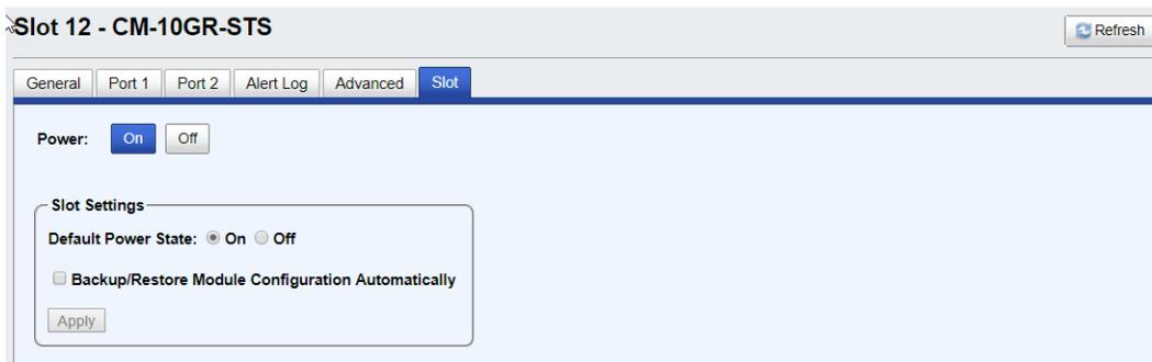
**Power State** Immediately power the slot on or off. The current state of the slot is highlighted in BLUE.
