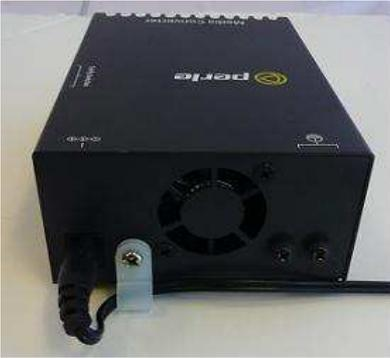
1. Feed the power cord through the opening in the power cord relief clip.
