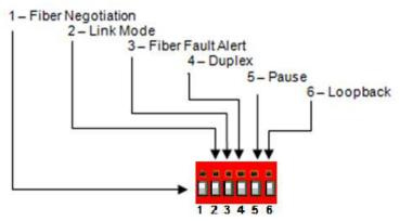
**Note**: Switch changes made when the product is powered up take effect immediately and will result in a link reset on both ports.
