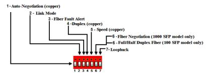
Note: All switch changes take effect immediately and will result in a link reset on both ports.
