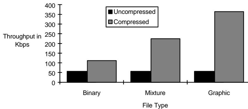
**Figure 1 - 6 Typical Throughput Over 56 Kbps Link**
