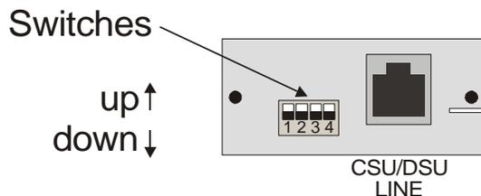
**Figure 3-1 Rear View of ATL-CSU/DSU Link Module Switches**
