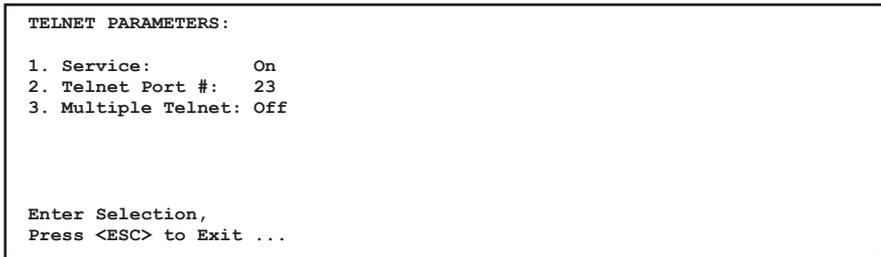
Figure 5.13: Telnet Parameters Menu - Text Interface
