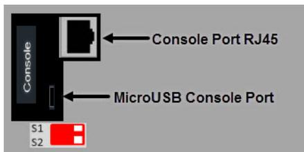
1. Connect an RJ45 cable to the IDS switch console port (RJ45) and the other end of the cable to a COM port on your PC.
