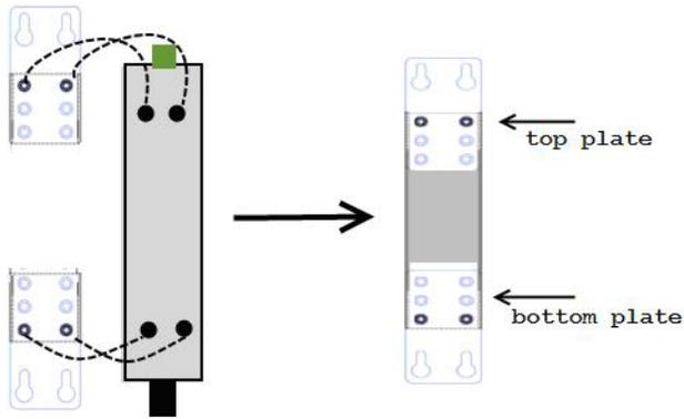
3. Use the wall mount plates as a guide to mark the spot where the screws will be placed.
