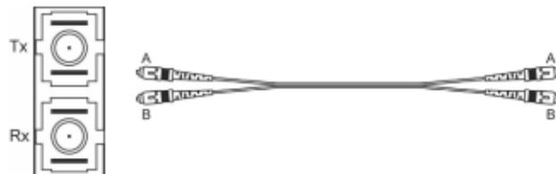
*ST-Port Pinouts*      *ST-Port to ST-Port Cable Wiring*
