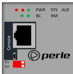
1. Connect an RJ45 cable to the IDS switch console port (RJ45) and the other end of the cable to a COM port on your PC.
