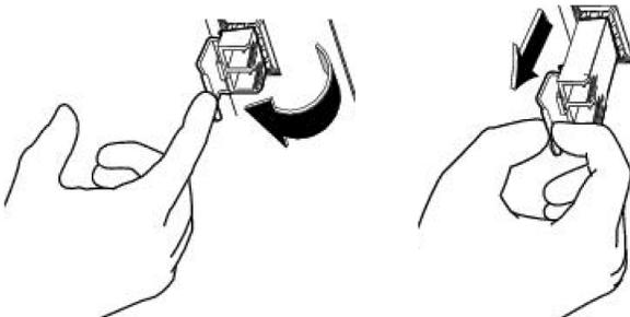
**Warning:** In hazardous location installations, failure to remove the power from the source prior to removing the SFP modules from their slots could cause an electrical arc resulting in a possible explosion.
