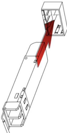
**Warning:** In hazardous location installations, failure to remove the power from the source prior to completing the connection/s to the SFP slot/s could cause an electrical arc resulting in a possible explosion.
