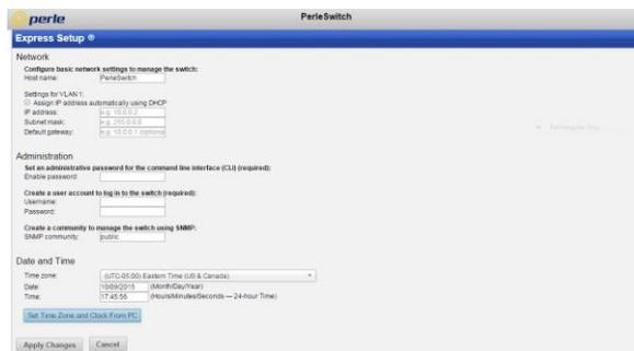
4. Once connected, fill in the required fields, apply changes to save and exit. The configuration changes will be immediately applied to the switch.
